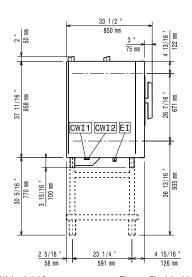
CWII Cold Water inlet 1 CWI2 Cold Water Inlet 2 ΕI Electrical inlet (power)
